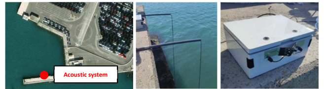
Fig. 7. Deployment of the system in Valencia Port and equipment prepared to work outdoors.
