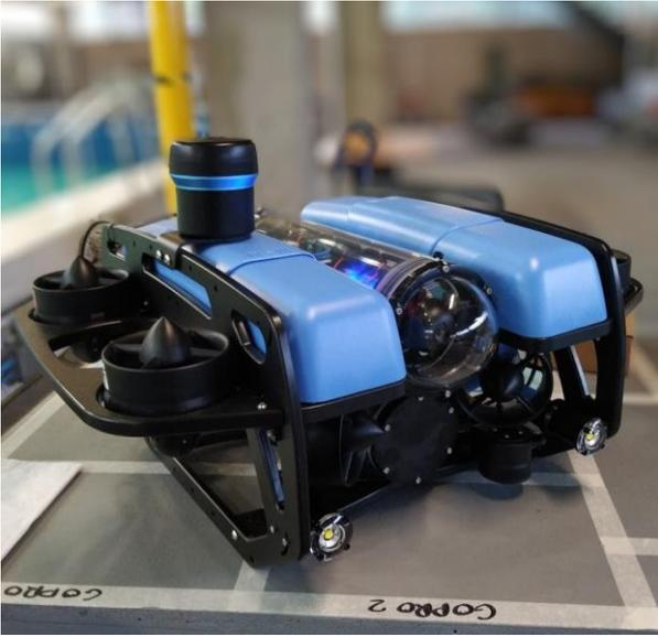
Fig. 3. BlueROV2 in its heavy configuration.
