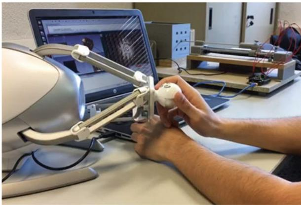
**Fig. 3** Novint Falcon, in foreground, with the robotic system and the phantom in background
