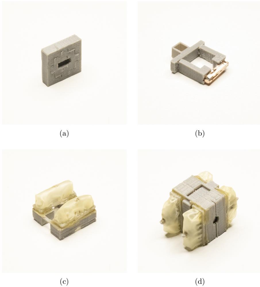
Figure 7: (a) Magnetic structure, (b) half of a tendon and the inner conductor, (c) linkage solution, (d) magnetic structure, tendons and inner conductor.
