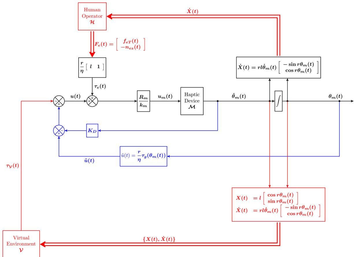
Figure 9.1: 1 DOF Haptic system with gravity compensation
