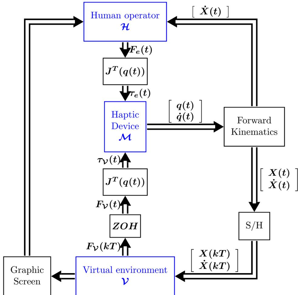
Figure 7.1: Block diagram of a haptic feedback.
