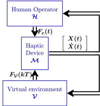
Figure 1.1: Block diagram of a haptic system.
