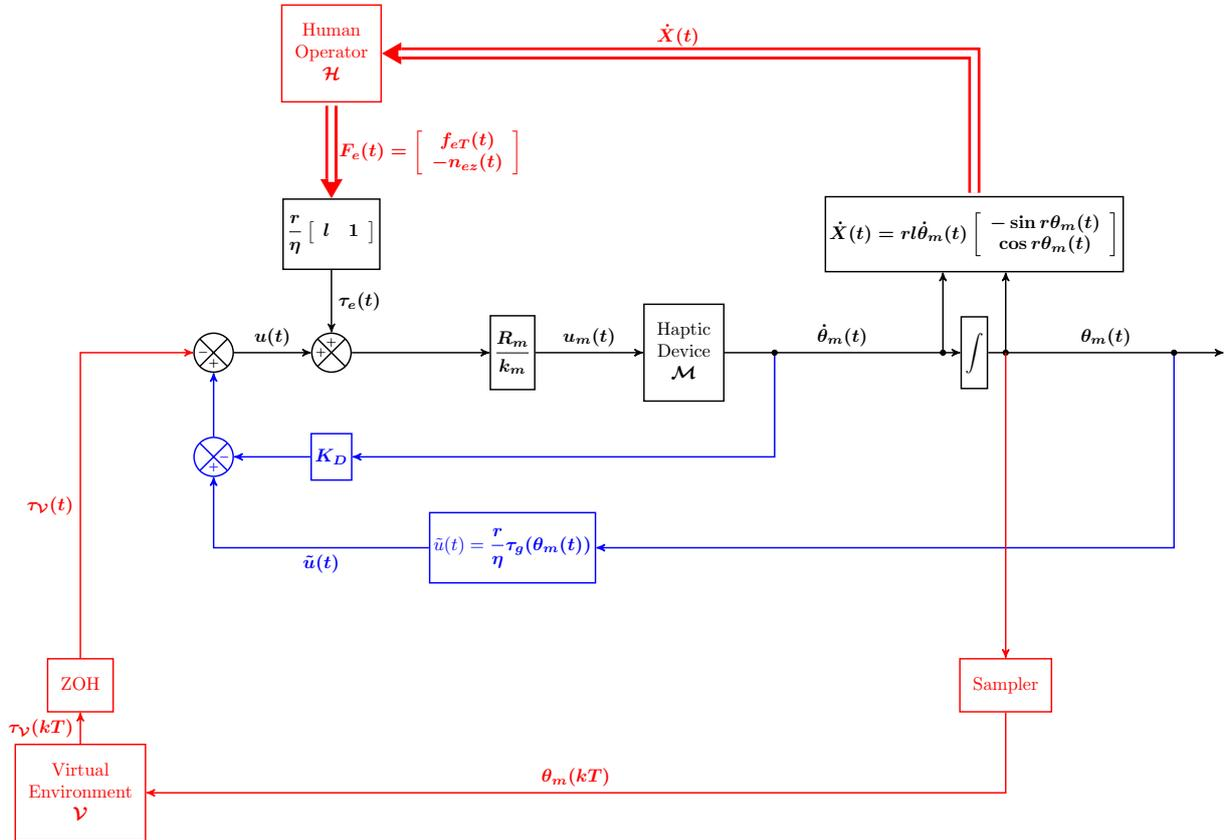
Figure 9.2: 1 DOF Haptic system with gravity compensation
