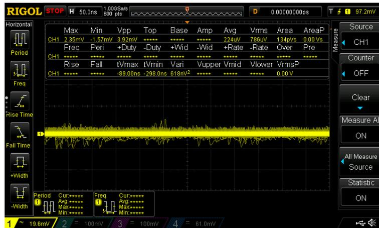
Figure 4.1: Noise measured on the analog +3.3V power rail.
