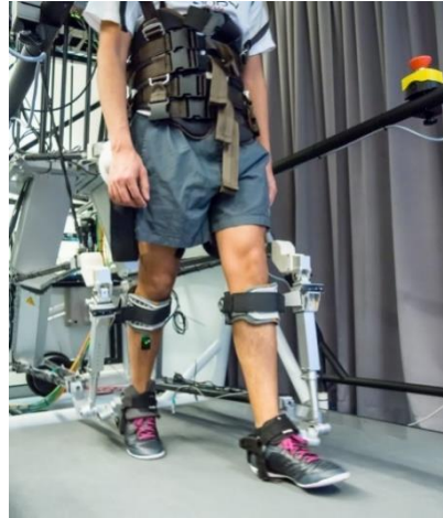
Figure 2.8: LOPES (Lower-extremity Powered ExoSkeleton) [23]
