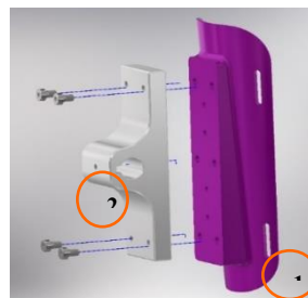
Figure 4.12: Subassembly of the extremity of the ExoLeg
