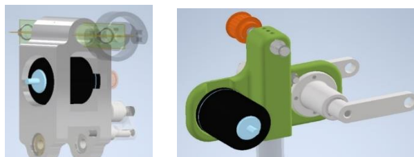
Figure 3.10: Motors integration to the design (motor 1 left, motor 2 right)
