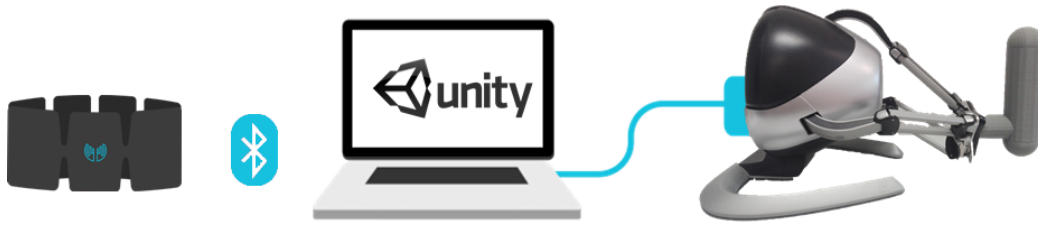
Figure 3.1: Schematic illustration of the rehabilitation platform, using a Novint Falcon, a Myo armband and a virtual environment.
