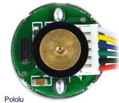
Figure 3.7 Magnetic disk and encoder, integrated in the gearmotor (Pololu, 2019).
