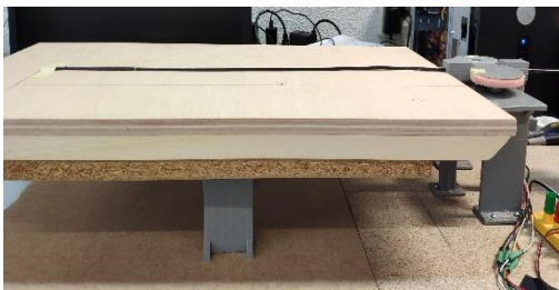
Figure 5.4 The cable located at the right height. It is the same height of the hole of the lateral support, that is the point from where the measure is performed.
