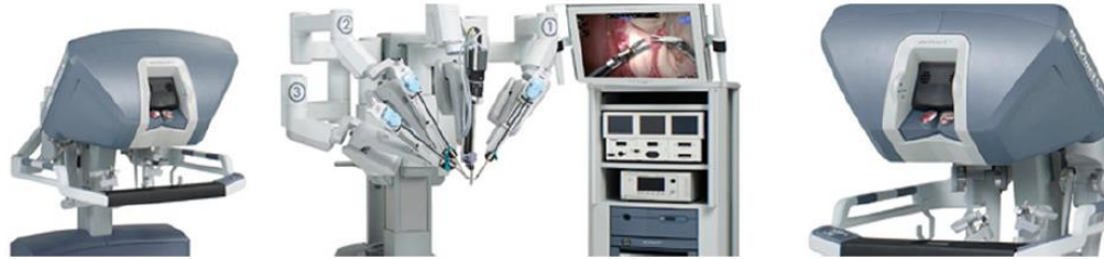
Figure 2.1 The components of DaVinci Surgical System (Intuitive Surgical Inc, CA, USA) (Simorov, Otte, Kopietz, & Oleynikov, 2012).
