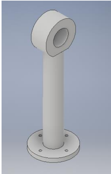
Figure 3.35 Support system cable-side. The instrument is inserted in the circle hole and can freely translate. It can be schematized in a cylindrical joint.
