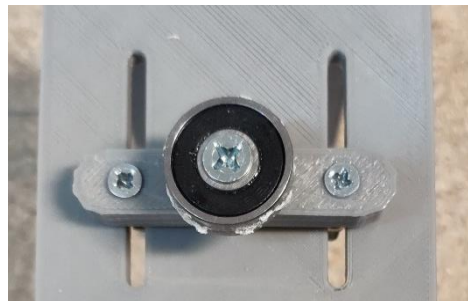
Figure 3.18 The system for the translation of the passive disk. It is possible to see the wheel that attaches to the disk. The well is fixed to a bar. At the extremities of the bar two screws are inserted. The two screws pass to the longitudinal slots of the support structure, allowing the system to translate.
