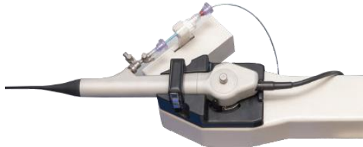
Figure 2.10 System for fixing the ureteroscope to the mechanical arm (Elmed, 2019).
