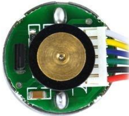
Figure 4.5 The upper part of a motor with the encoder and all the cable needed for motor management (Pololu, 2019).
