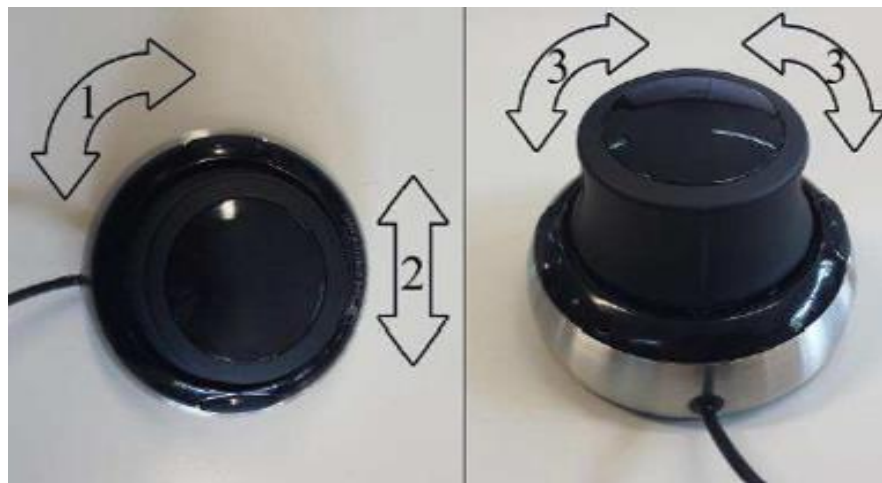
Figure 4.8 The movement of the 3Dmouse used to perform the system motion. 1: rotation of the cap to rotate the ureterscope; 2: Back and forth inclination to insert and retract the cable; 3: Right and left inclination for the tip deflection.
