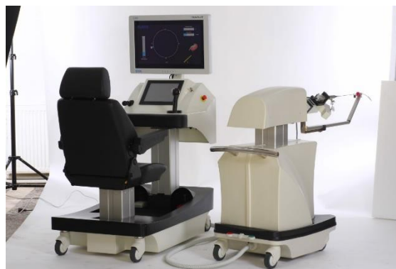
Figure 2.9 Last version of Avicenna Roboflex (Elmed) system, with the left horizontal joystick for insertion and rotation, and right joystick for deflection control (Roboflexusa, 2019).
