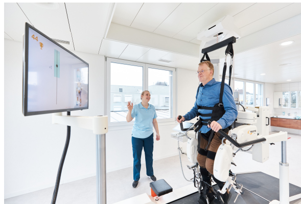
Figure 2.4: Lokomat orthosis, image retrieved from Hocoma web page [32].
