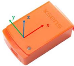
Figure 4.2: XSens IMUs reference system. Retrieved from [41]
