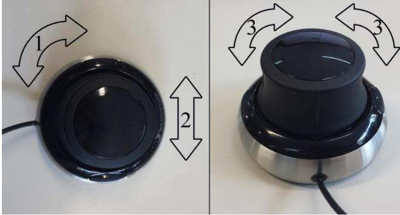
Figure 2.4: 3D mice used as endoscope controllers. On the left, 3D mouse for the left hand controlling rotational motion (1) and insertion motion (2). On the right, 3D mouse for the right hand responsible for flexion motion (3).
