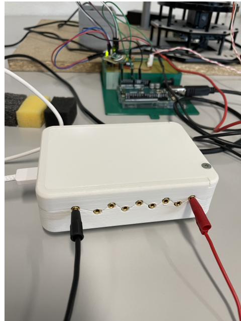
(b) Red banana cable connected to channel 1 for stimulation and black banana cable connected to the EAST reference.
