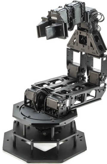
Figure 3.8: PhantomX Reactor Robot used to mimic the functionality of an upper-limb prosthesis
