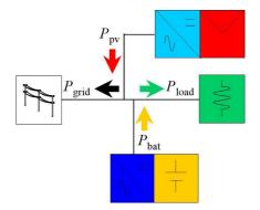
**Figure 1:** Block diagram of PV hybrid system installed in a typical grid-connected building.
