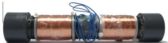
Fig. 1. Kinetic generator in secondary nodes.
